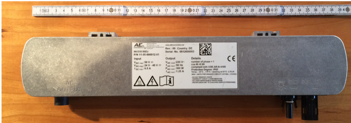
Figure 2: Microinverter made for the project to fit into the rail system of the balcony.
